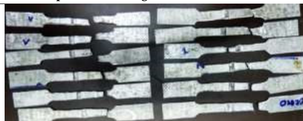
Figure no.11 fractured sample after strength test
