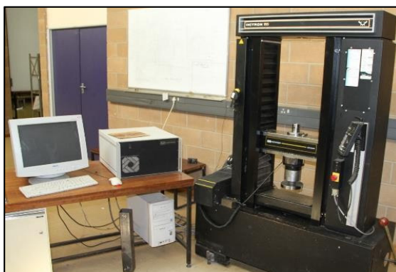
Figure 7: Instron 5500R electromechanical tensile testing machine used
