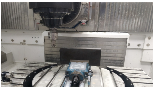
Figure-1: Side milling of the workpiece on 5-axis Milling machine
