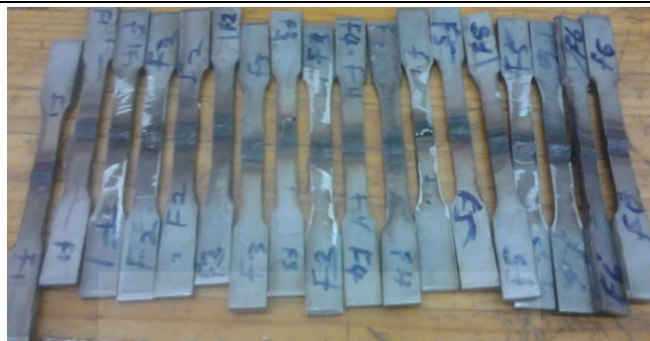
Figure 16 : Samples prepared for tensile test
