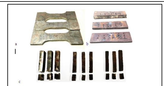
Fig. 3. Pictorial representations of (a) Tensile Test; (b) Hardness; (c) Izod Specimens
